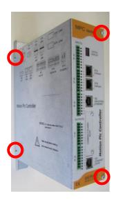
a – You must begin by disassembling the front cover, remove the 4 fixing screws.
