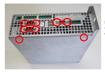
b – You must remove the grill from top, remove the 2 fixing screws and 6 columns.
